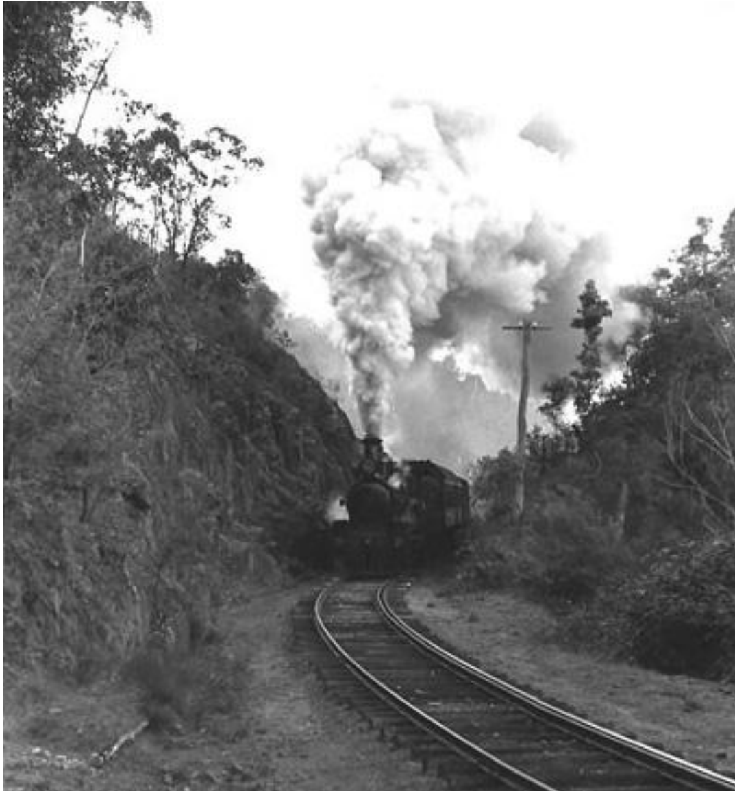
Figure 3: A hard-working 19 class loco climbs the 1:25 grade towards the summit with the Oberon mixed on its way from Tarana to Oberon – note the sharp curves with checkrails and essentially unballasted sleepers. (© Dennis O’Brien collection).
