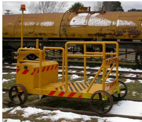
Officially known as an Emergency Response Vehicle (ERV) it was used as a track inspection vehicle or a people mover during track maintenance. In emergency situations it was equipped to carry stretchers. The vehicle is battery powered.
