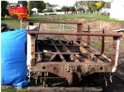
the old wagon stripped down prior to being sandblasted in preparation for the repainting of the steel framework. Quotes for timbers compatible with the originals have been received and will shortly be on site. We now look forward to seeing the work develop. Keep watching this space for more progress photos as the project continues.
