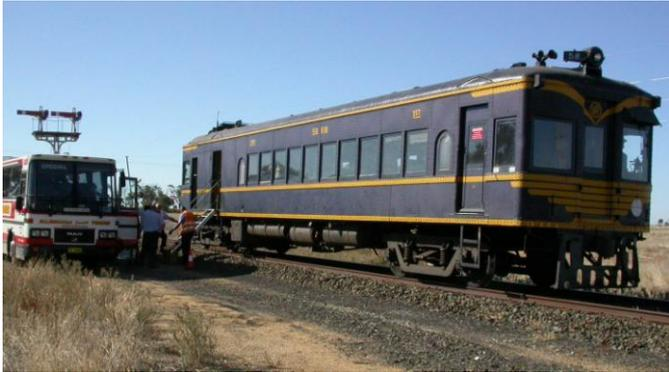
The DERM is unusual in that the two GM diesel engines and generator are above the floor at one end of the railmotor. The luggage area separates the engines from the passenger seating. The unit may be driven from either end. It holds 58 passengers and is equipped with a toilet. The interior shown below has fixed seating with varnished timber panelling. These are capable of 100km/hr – as was demonstrated on this tour.
