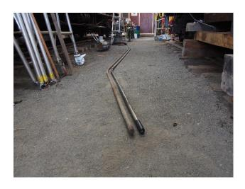
New truss rod alongside the old. The old one had thread damage and the engineering report indicated the diameter had narrowed too much
