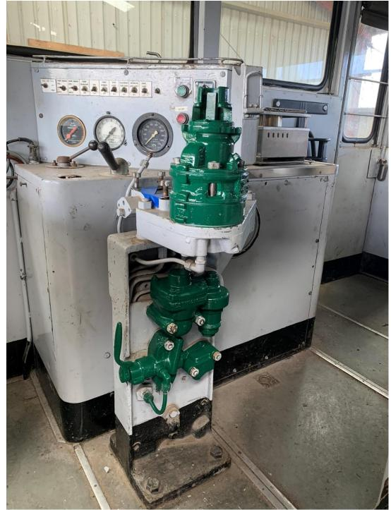
Newly serviced and installed in locomotive 7321 AH7 automatic brake valve, M3 feed valve, isolating valve and equalizing reservoir control valve
