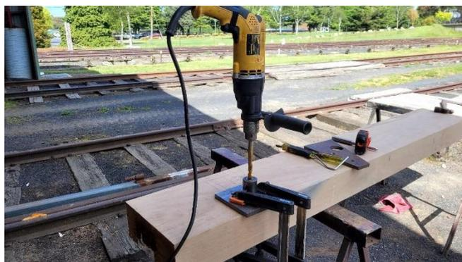
*Preparing to drill holes for the guard's end headstock of HLF854*
