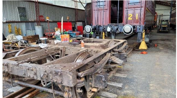
Set of bogies rolled out for inspection.
