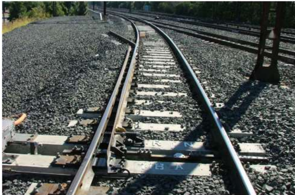
Figure 4 – Example of catchpoint with good landing zone
