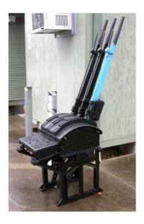
Three lever ground frame donated by Garry Leamey, State Rail Signals Engineer for Blue Mountains. Garry has been a great help in sourcing bits and pieces like this lever frame to help with the restoration of the Oberon line. The frame is in great condition having recently been repainted and now retired from active service.
