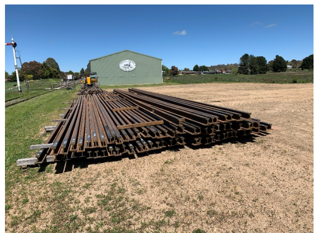
1 km of 80 lb rail neatly stacked and ready for use
