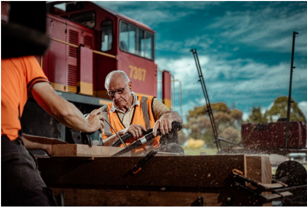
Another angle of the making of headstocks for our End Platform Carriage against a lovely Oberon Summer sky.
