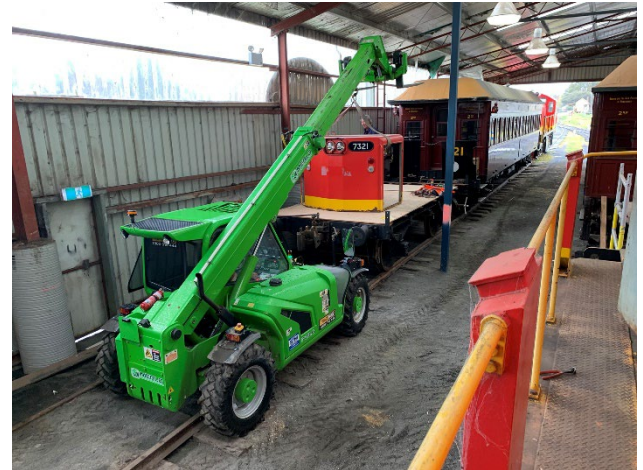
Removing body of Locomotive 7321 in readiness for its restoration. Rolling Stock Manager Mark Handel in the background. Photo also features the interior of the OTHR Rolling Stock shed.
