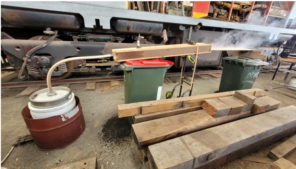
Steamer for bending guard wall matchboard.
