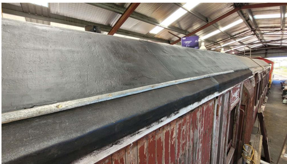
Roof side bitumised. First aluminium holding strip re-installed over gutter line canvas.
