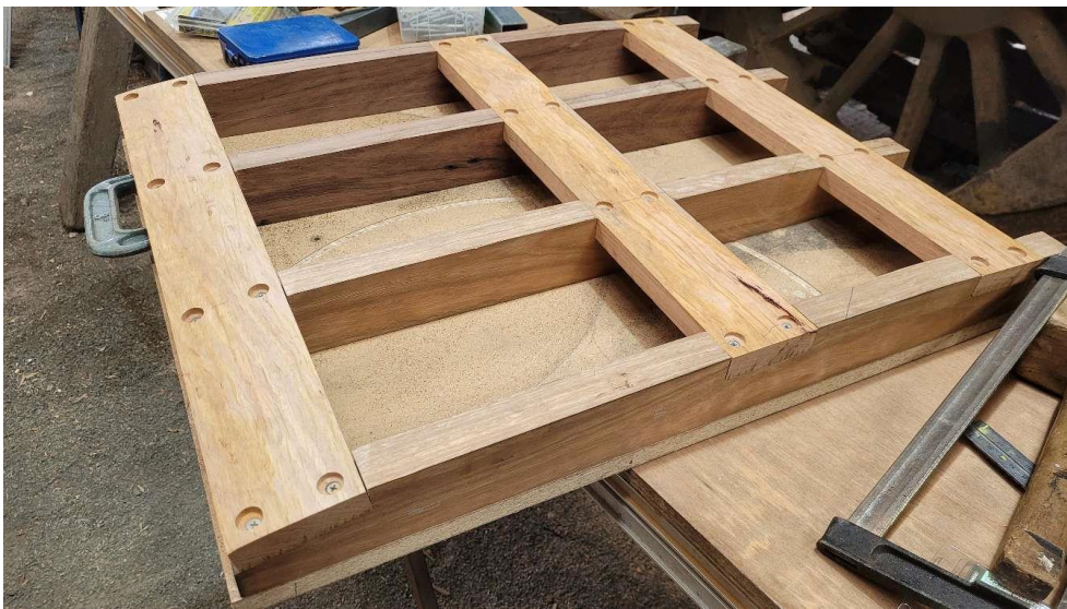
Bending buck made replicating lower wall section. Used for steam bending.
