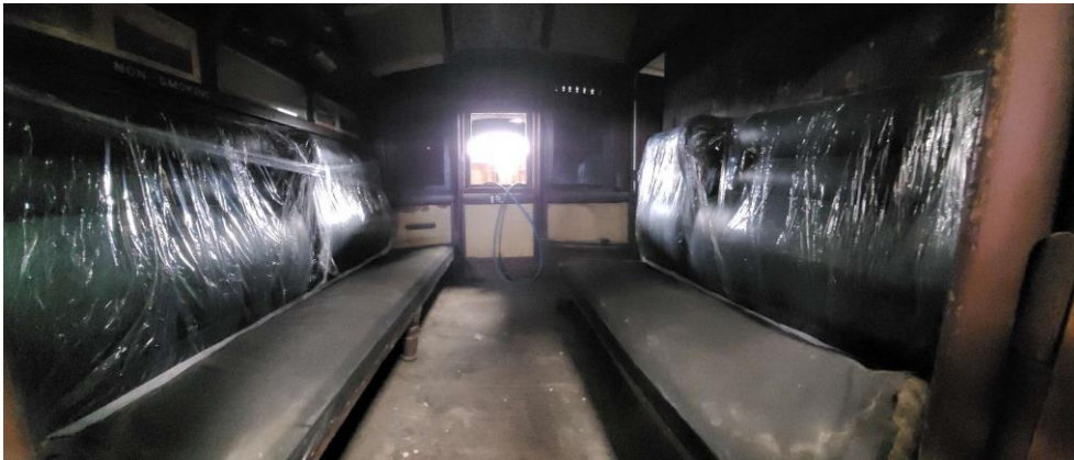
D36 first class finished seat backs temporarily placed for seat base measurements.
