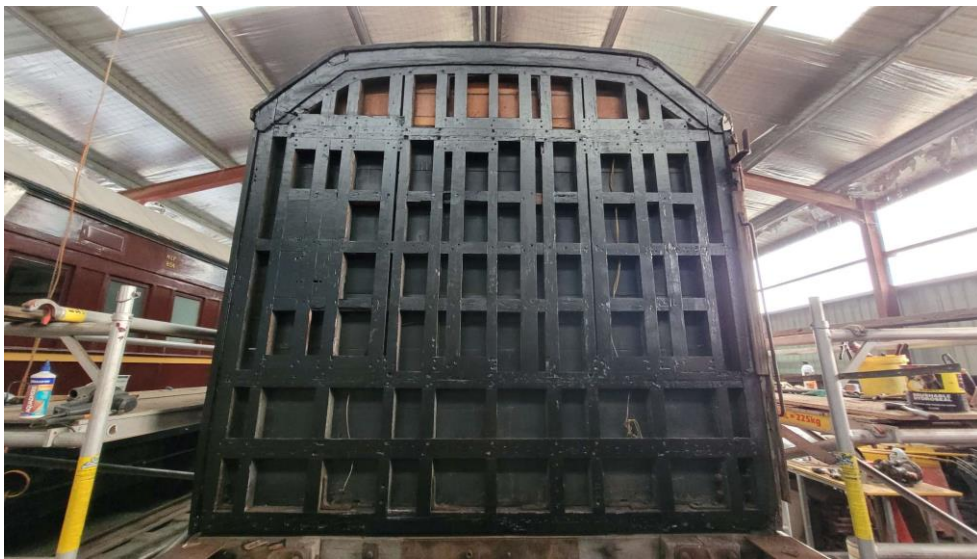
Frame repaired and painted ready for matchboard. Guard end.
