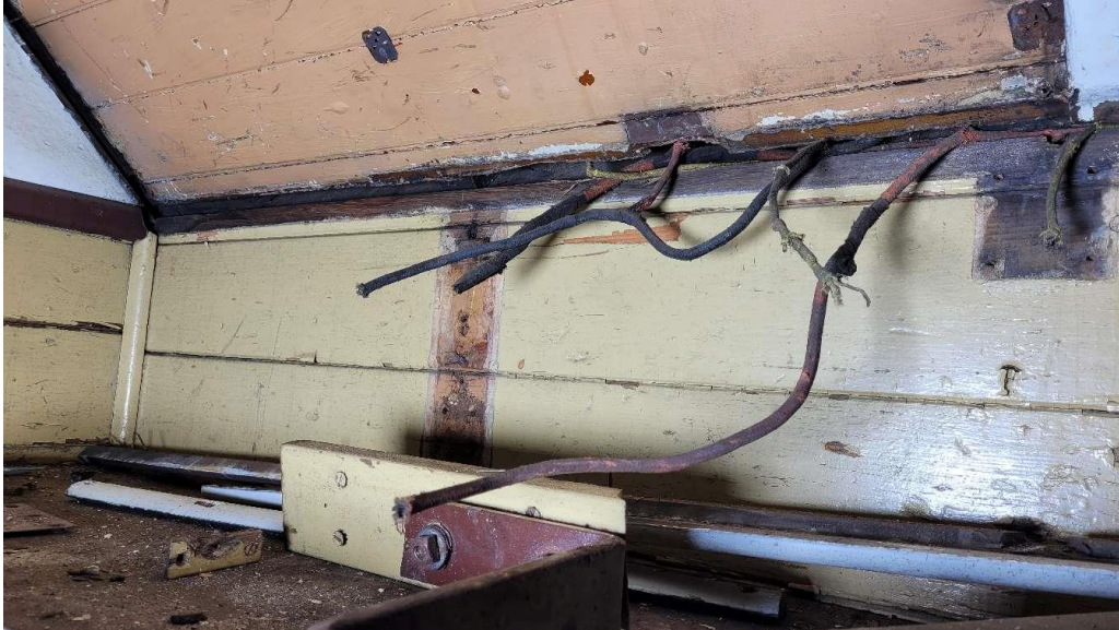
Old wiring (already cut) in guards' compartment.
