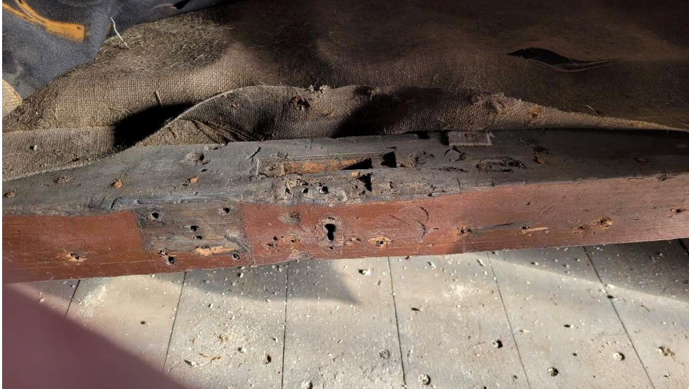
Original linen mortise lock in seat base of D36 compartment upholstered over.
