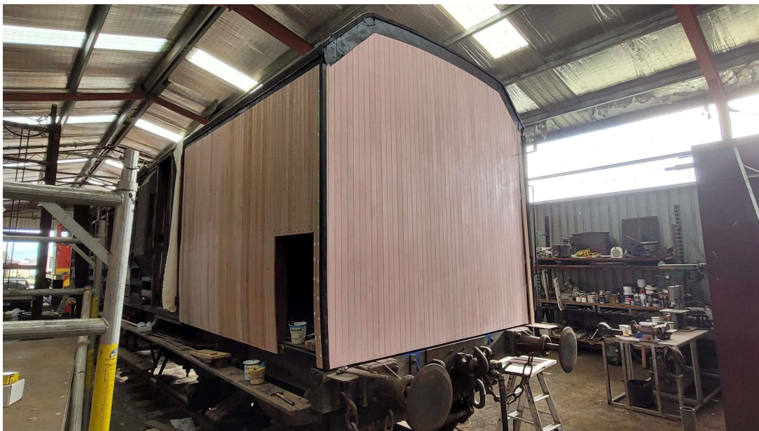
Guard wall application showing dog box door cavity.
