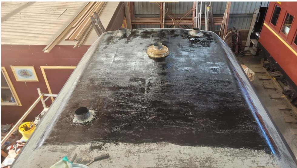
Guard end roof sanded and bitumen applied. Cracks filled. Repaired centre vent installed.
