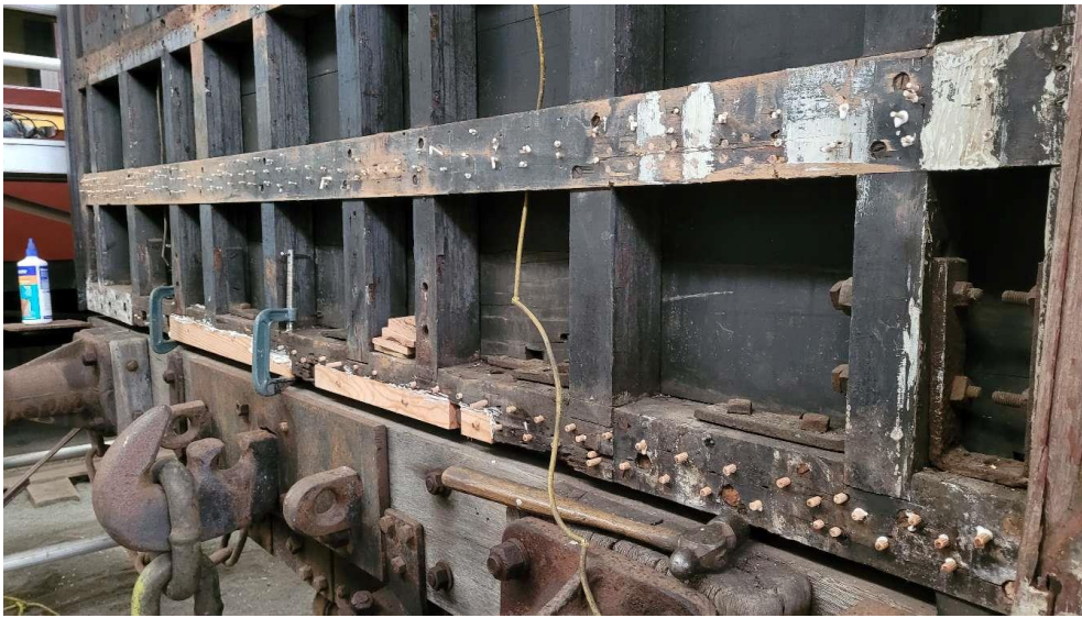
Rot repairs completed. Screw and nail holes dowelled.
