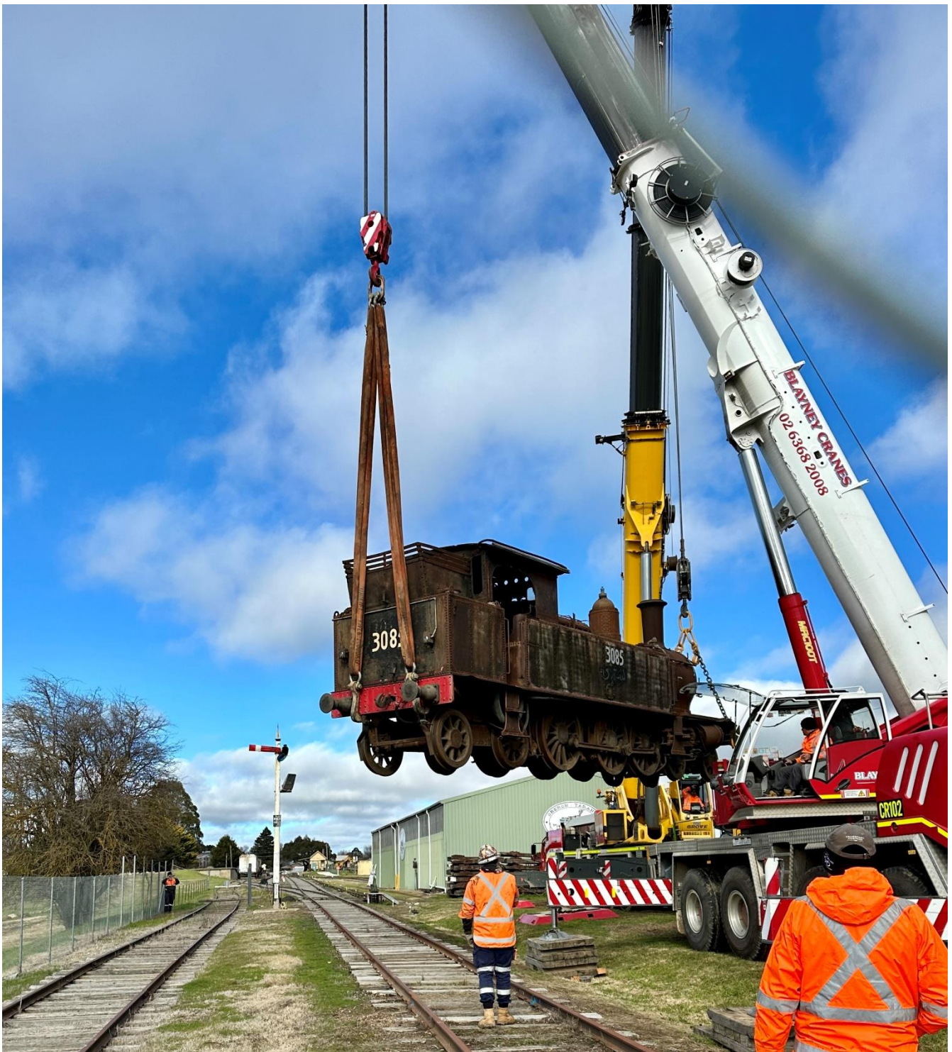
Careful movement to lower 3805 onto the rails
