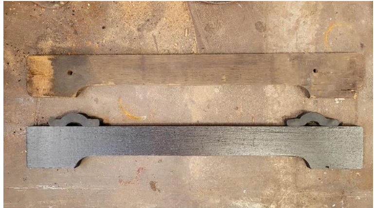
New drop light timber support bars made with new rubber bumpers in place.
