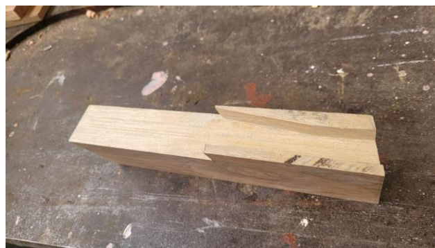
New tallowood for frame repair
