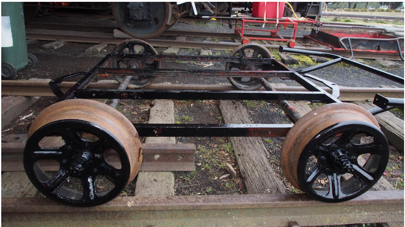
Frame of the Light Ganger's Trolley LGT 348 has been painted, grease nipples on the axles have been serviced
