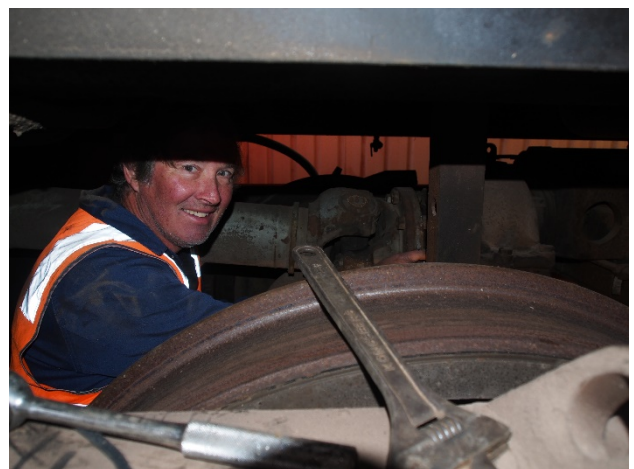
Mark Handel checking the Carden Shaft Bolts and Oil Levels in the Differentials
