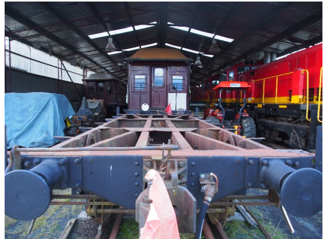
Undercarriage of the cattle wagon which may have to be used as a match wagon in the future. Recent work has been removing rotting timber work and straightening bent metalwork
