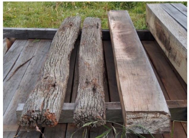
A couple of very old sleepers along - side a new one. They were recently removed from Road 3. They are split at the end; the dog spikes were loose and would not have been holding the track in gauge. How long were these in the line?
