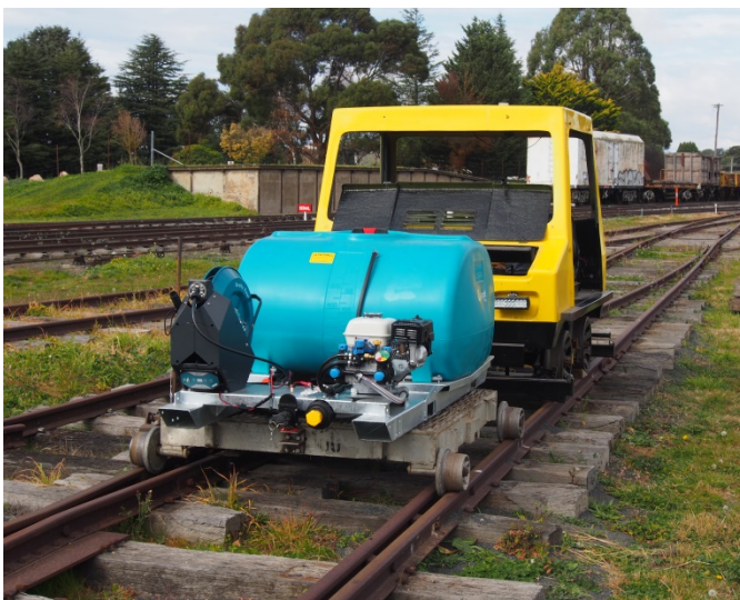
The new spray unit mounted on a sleeper trolley. This will be very useful as we do track maintenance north of Albion Street.
