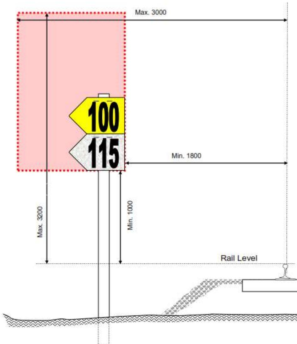
Figure 12 - Placement envelope for permanent speed signs
