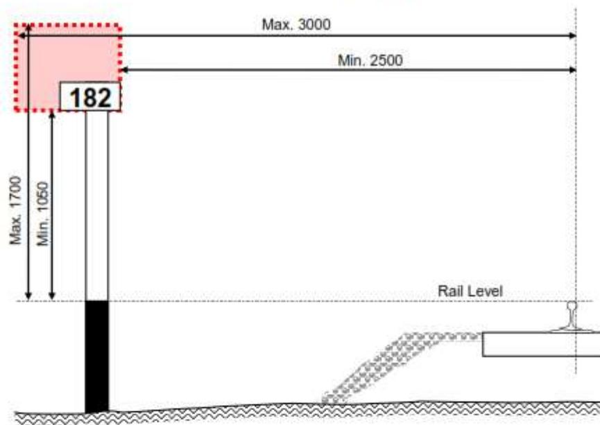
Figure 16 – Lateral placement of kilometre posts
