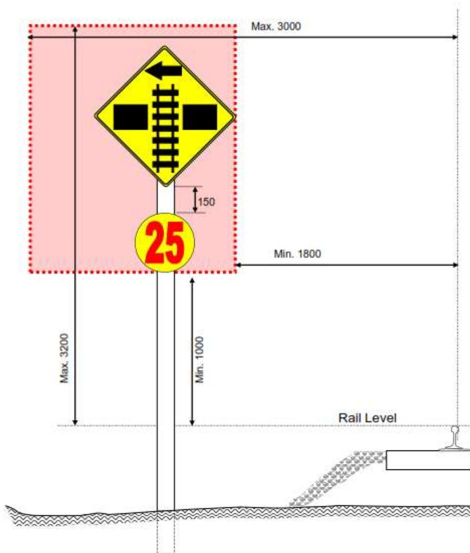
Figure 14 - Placement envelope for conditional level crossing speed signs
