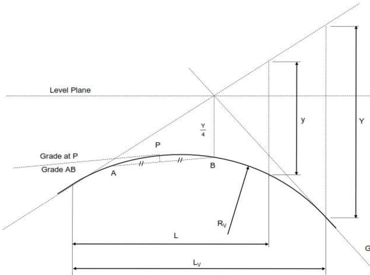
Figure 9 - Vertical curve component
