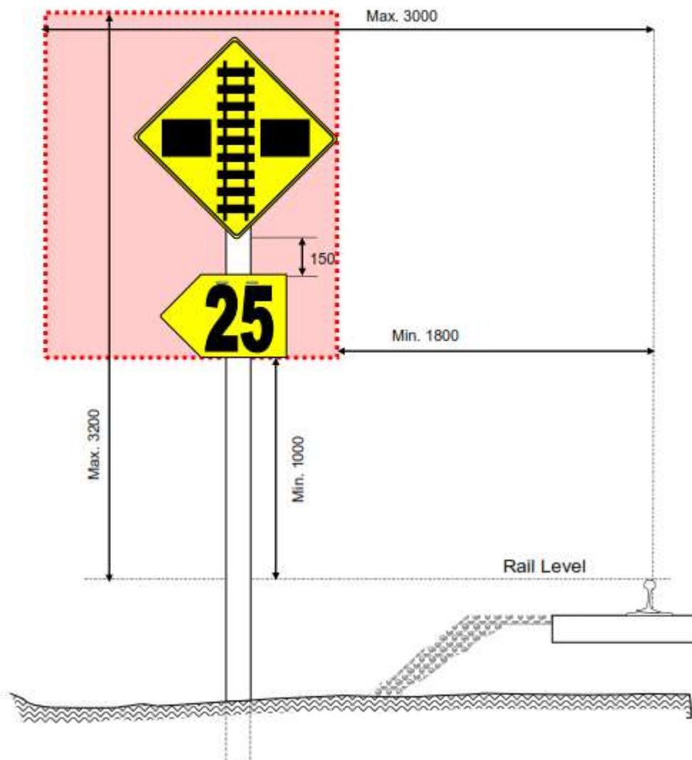
Figure 13 - Placement envelope for level crossing speed signs
