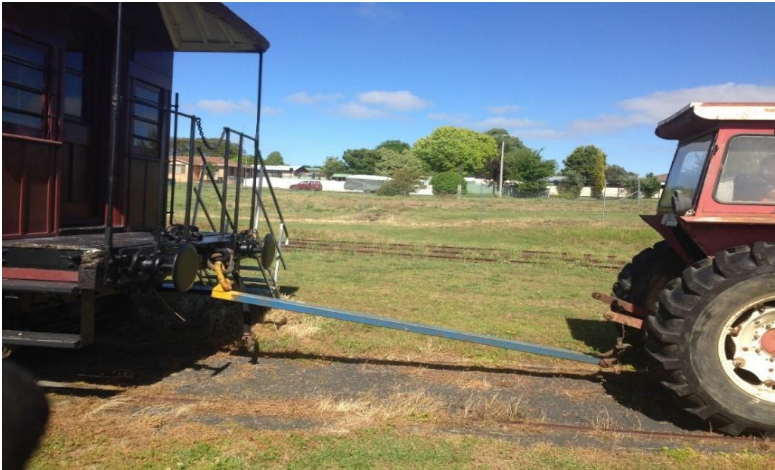
Example of coupling the tractor to an End Platform Car
