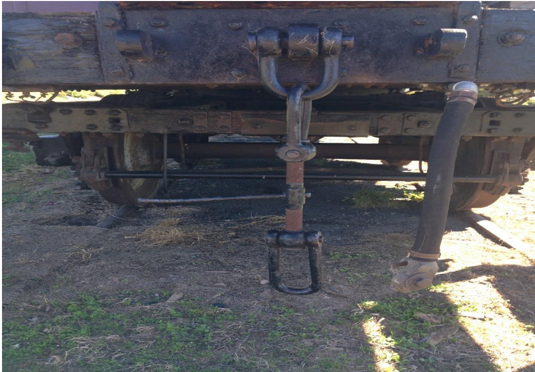
The link is connected to the hook on the other vehicle
