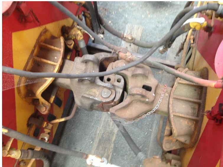
An example of two vehicles connected to with auto couplers
