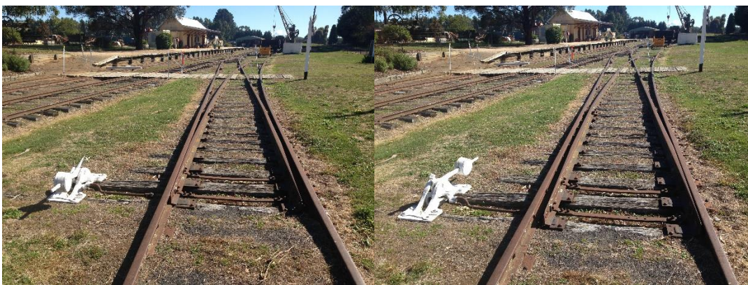
Points changed by a 'Throw over' lever
